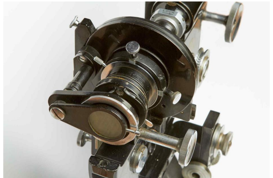
The model 47 microscope is equipped with remote coarse & fine focus (drive band missing from fine focus pulleys)
