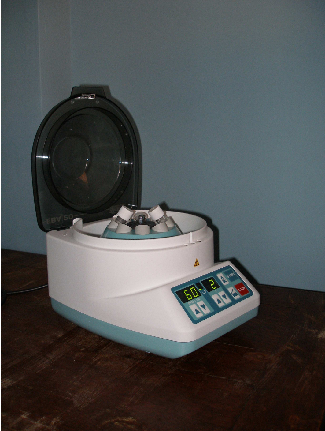
Figure 2: Small centrifuge with fixed angle rotor
