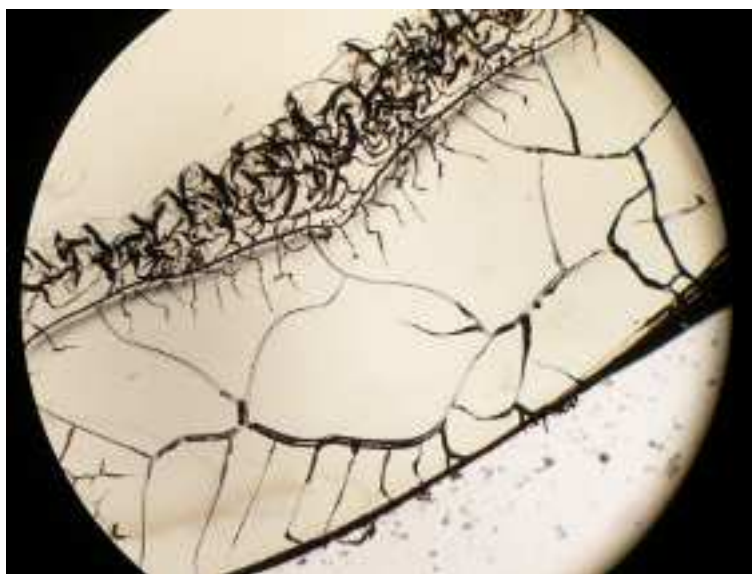
Figure 2: Detail of crazed resin
